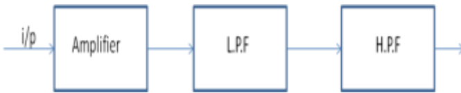
Fig. 2 Block diagram of the filter
